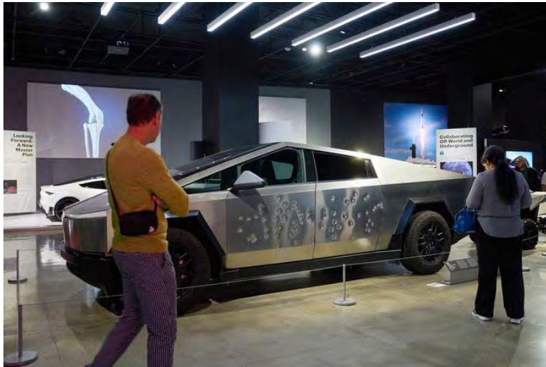
A Tesla Cybertruck prototype that was used in bulletproof testing. PHOTO: ALLISON DINNER/SHUTTERSTOCK
